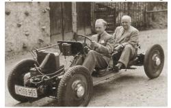
Hans and Jorge Rasmussen drive the Framo-Goritz streamliner chassis. Although space age in appearance it remained a budget car. The car's single cylinder, 200cc water cooled two-stroke engine is clearly visible in the photo.
